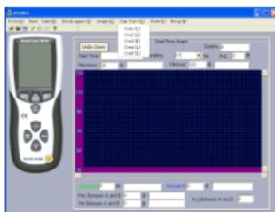
1.5 Enter the menu REAL TIME\ 'SETUP' to set the monitoring data(data volume, response, monitoring time)
