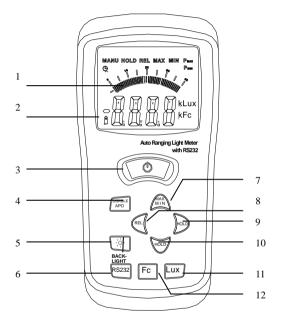
LCD Display: 3-3/4 digit displays with a maximum reading of 3999, and the indicating signs of measured values, unit function symbols and decimal points etc are display.
